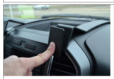
3. Press down on the face plate of the ProClip to make sure the tape adheres to the dash
