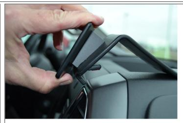
2. With your finger behind the face plate of the ProClip, flex the thick angled edge on the back side of the ProClip out and around the dash, then insert the edge into the top of the right center vent opening.
